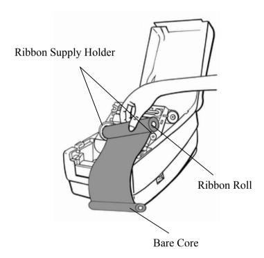
7. Turn back the print head module and then insert the bare core into the pick-up holder.(first snap in the left side, then the right side)
